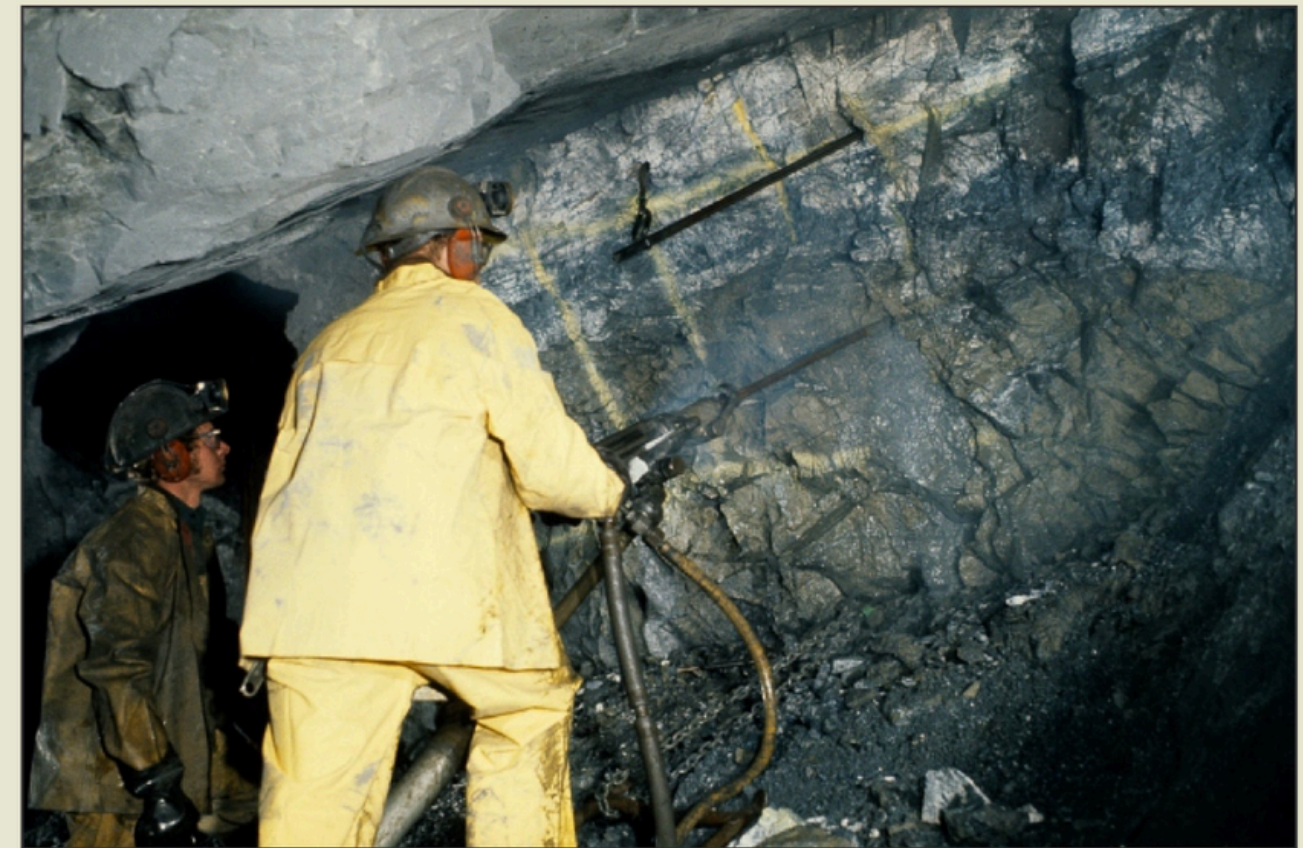
Underground mining of the antimony vein at the Lake George mine.
